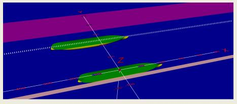
ships and wind. The potential code ROPES was first used to calculate the passing ship forces, which were then put in the software Vlugmoor, which has been developed specifically by the Division of Maritime Technology for Dynamic Mooring Analysis. Not only mooring line forces, but also motions of moored ships need to be limited, as large motions can cause delays and potential safety risks.
