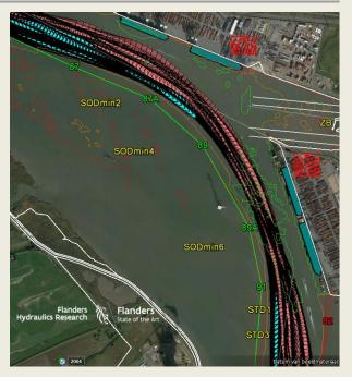
(sim360+ and sim225) for the evaluation of an optimised Europe terminal layout. In this optimized orientation, ULCC encounters and swinging manoeuvres were studied. The pilots passing by moored MM24 ships at the optimised Europe terminal adapted the speed through water and passing distances in order to guarantee a safe passage. The simulations were executed in strong wind conditions of 5 and 6 Bft and with maximum current during flood or ebb tide.
