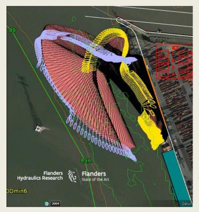
For the swinging manoeuvres in the vicinity of the Europe terminal, ULCCs of up to 430 m were handled by pilots of both the Flemish and the Dutch Pilotage and by tug captains of Antwerp Towage and Boluda during the simulations at <u>Flanders</u> Hydraulics Research.
