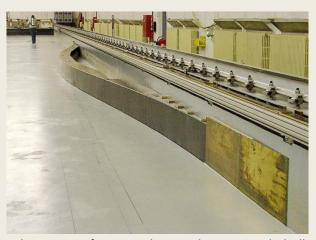
The mathematical model was validated by studying the transit of a 230 m long and 37.5 m wide bulk carrier on the Canal Ghent-Terneuzen with both Dutch and Flemish pilots. In 2016 a new experimental program will be carried out in the towing tank to study additional transient bank effects.
