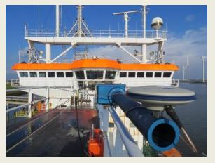
In order to assess the influence of a <u>nautical</u> <u>bottom</u> in the port of Delfzijl, the Knowledge Centre carried out four <u>full scale trials</u> to measure the motions at full scale of the hopper dredger Geopotes 15 (Van Oord Nederland bv). During these trials a wide range of tidal levels and bottom conditions were experienced, corresponding to under keel clearances with respect to the top of the mud layer varying between +17% and -5%.
